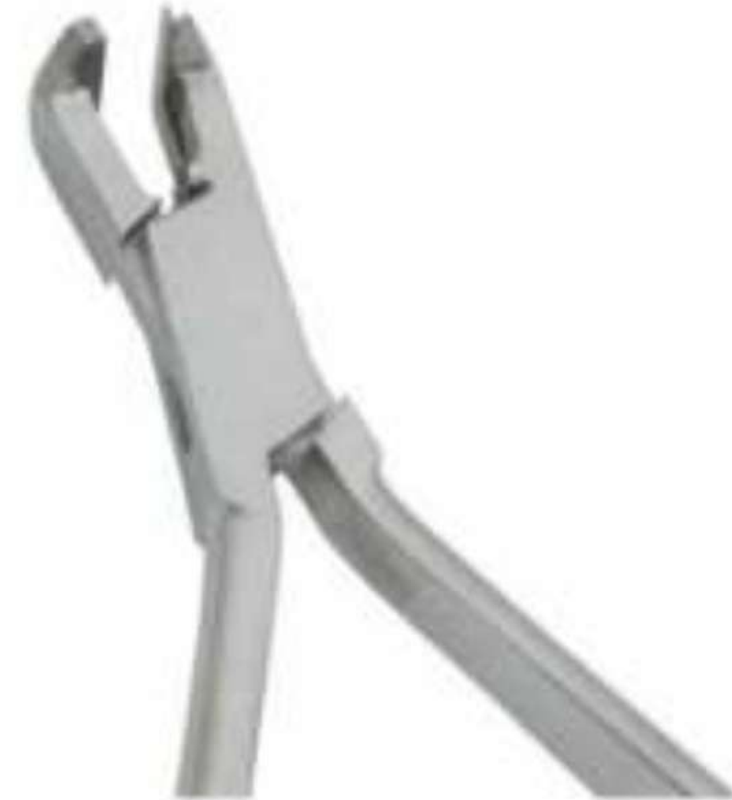
BI-5-003 1-Distal End Cutter Flush Cut with Safety Hold This instrument cut wires close to the buccal tube and safely holds the distal end. The tungsten Carbide insert ensure precision cutting, long wear and unsurpassed cutting performances. Maximum Cutting Capacity. arch wires up to .021"x.025"(.55mx.64mm)
