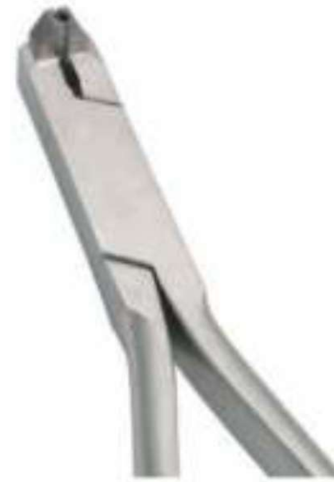
BI-5-005 1-Distal End Cutter Flush Cut This instrument cut wires close to the buccal tube and safely holds the distal end. The tungsten Carbide insert ensure precision cutting, long wear and unsurpassed cutting performances. Maximum Cutting Capacity. arch wires up to .021"x.025"(.55mx.64mm)
