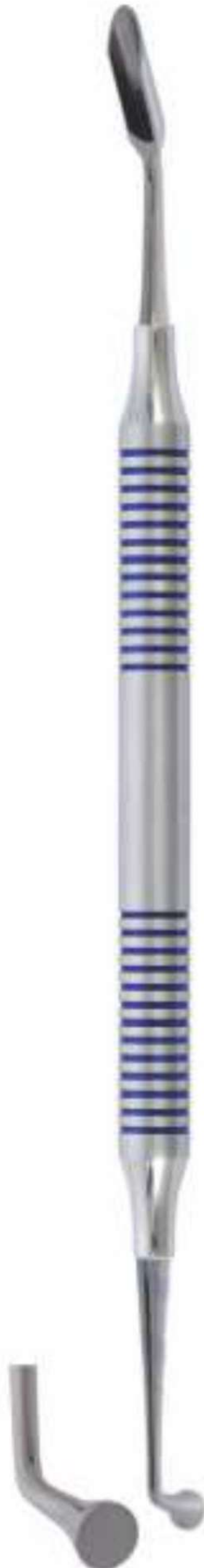
BI-6-100 Blade and pusher Length 180 mm, for straight or angled, blade: 15 x 5 mm, pusher: 4 mm diameter angular
